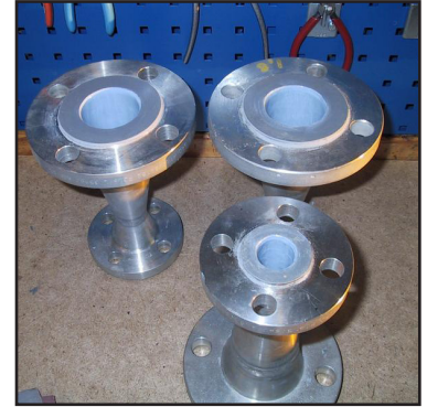
Individual small bore nozzle coating
