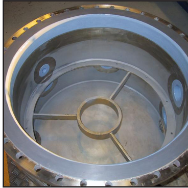
Vertical view showing protected flange faces
