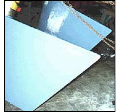
Both stabilizers completely rebuilt and coated.
